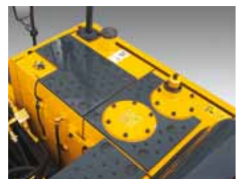
Anti-Slip Plates on Upper Structure
